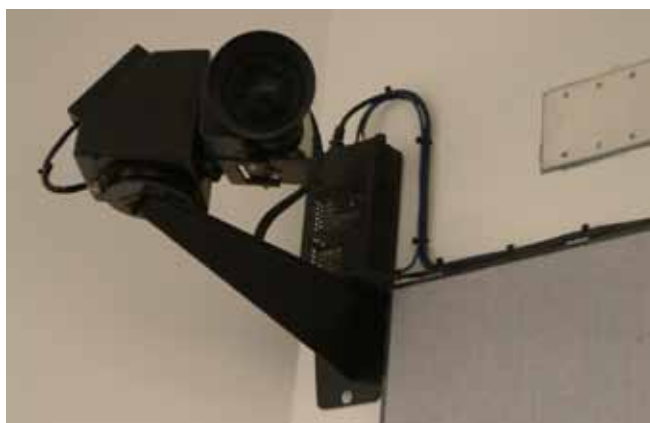
A PTZ camera mounted high on a wall.
