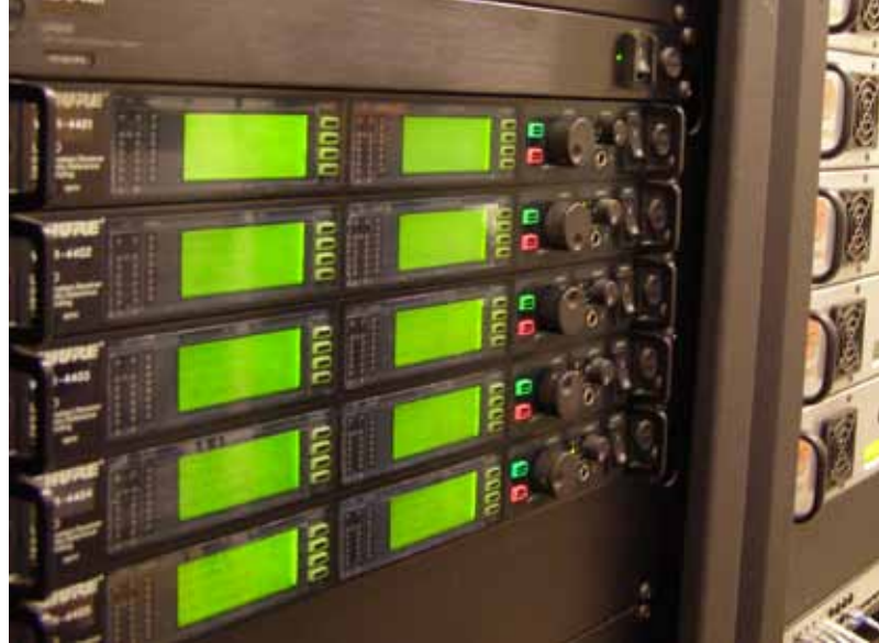
A group of 10 wireless microphone receivers in an AV rack.
