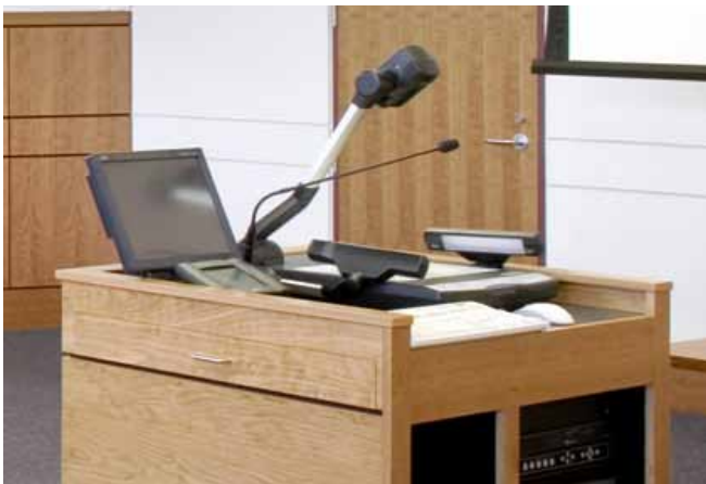
Presentation lectern with monitor, small control touchpanel, evidence camera, and microphone.
