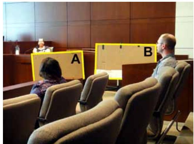
Example of a sightline mockup test for jurors. View is looking toward the witness from the third row of the jury box. Note the very poor view of the "A" monitor.
