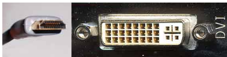
An HDMI connector; a female DVI connector.
