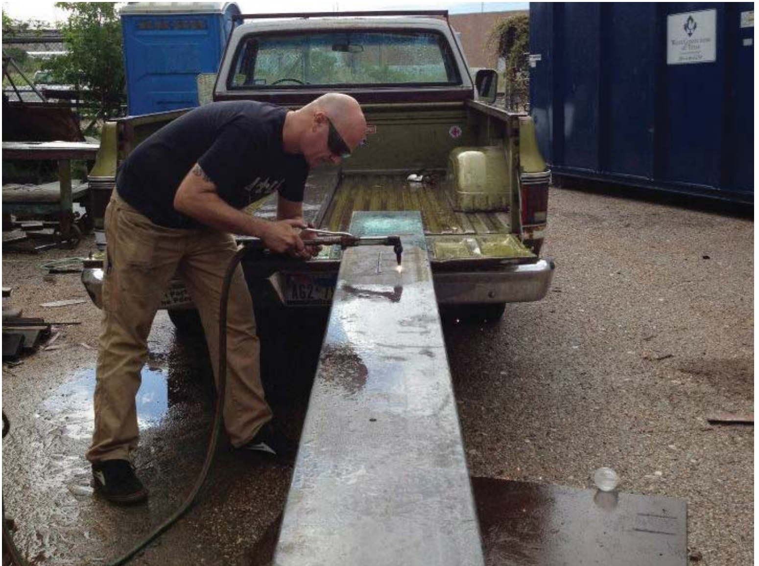
STEEL FABRICATION : THE PROTOTYPE WILL BE BUILT ON THE TRAY SO THE FORKLIFT CAN LIFT IT
