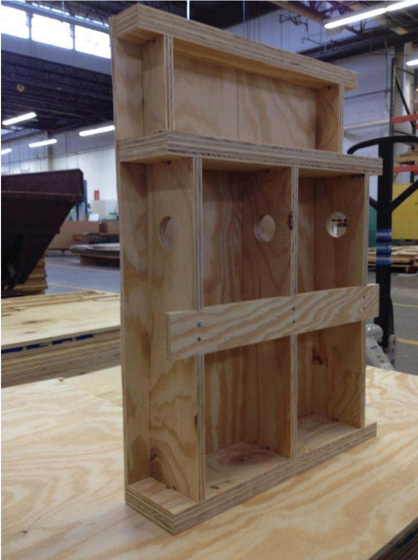
MOCKUP : MOCKUPS TESTED THE JOINTS AND CONNECTIONS OF THE STRUCTURAL PLYWOOD SYSTEM
