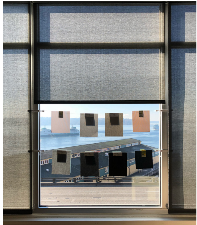
Using make-shift 3D printed clamps, DLR Group tests pre-validated PVC-free shade cloth options. Photo by DLR Group.
