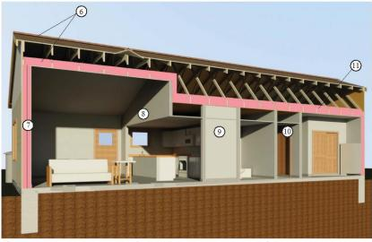
6 Roof Truss with Energy Heel
