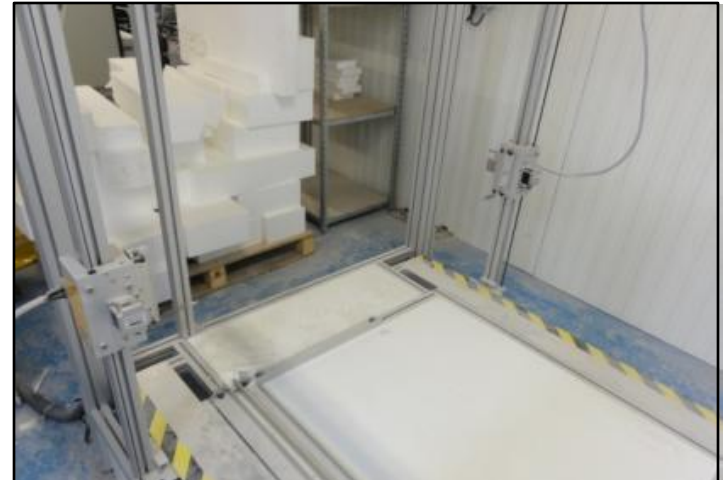
Hot Wire Cutter – for ruled surface panels
