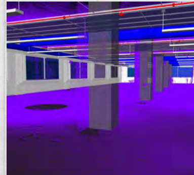
Navisworks image showing point cloud vs. architectural model; Note the differences in column locations
