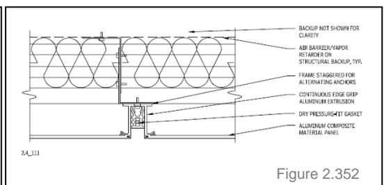
Mounting typically falls into either exposed or concealed fastener types. Whichever fastener type, ensure that the
