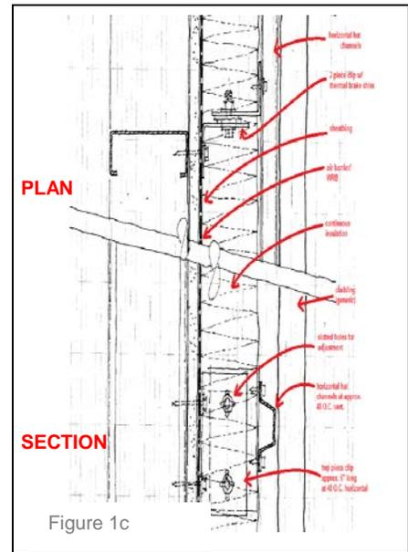
**Cladding:** The outer cladding of the wall assembly can be a wide variety of materials. For the sake of clarity this layer is not referred to as the “rainscreen”. This name has created confusion and seemingly led to the idea that the cladding can be nearly anything, including open jointed systems, perforated materials, and literally screens. The cladding must be detailed to attempt to stop ALL water intrusion to qualify as a proper BVDC or PER system.
