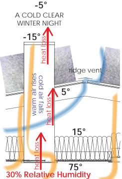
The tube is not carefully sealed. Air can easily enter the tube at the bottom and at tube joints within the attic. The tube is a heat transfer machine (in this case 90°  $\Delta T$  from the top to the bottom). Inside the tube, air carries heat from the bottom to the top by convection. The metal of the tube is constantlypulling heat up and out. Much of the tube is at a temperature below the dew point of interior air, so condensation is occurring both inside and outside of the tube.
