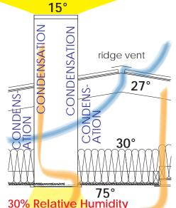
The dew point of 75° at 30% relative humidity is 39°. More or less, all of the tube that is above the top of the batt insulation is below the dew point. Any warm interior air that manages to get into the tube or into the attic will condense moisture onto the tube. Much of the tube is well below 32° and thus much of this condensation will be stored as ice.
