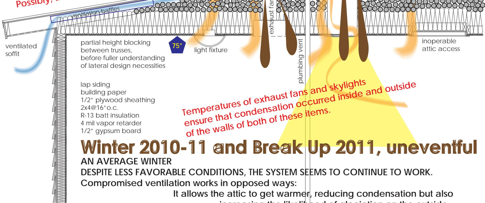
*Temperatures of exhaust fans and skylights ensure that condensation occurred inside and outside of the walls of both of these items.*
