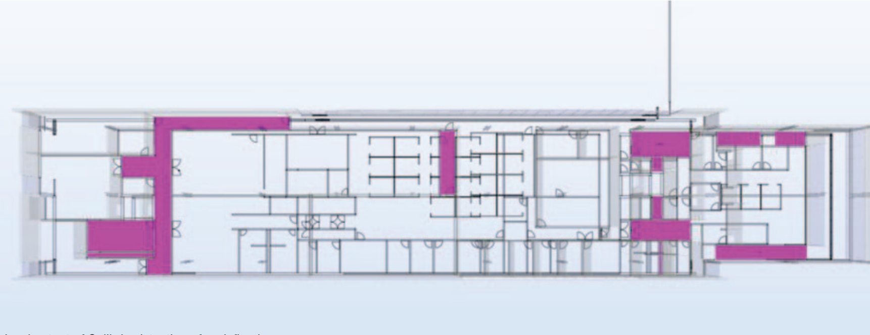
visual output of Solibri - detection of undefined spaces
