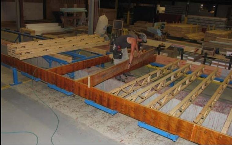
4" Foam blocking on outside perimeter of floors – open web joists – urethane adhesive on floors
