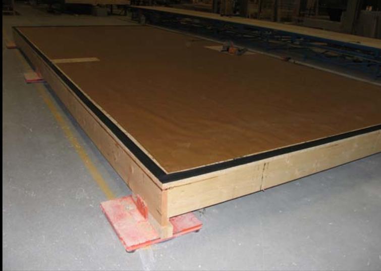
EPDM gasket at floor and wall intersections
