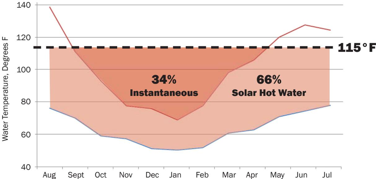
The New Norris House utilizes a solar hot-water panel system made by Enerworks. The system is supplemented by a small Eemax instantaneous water heater.
