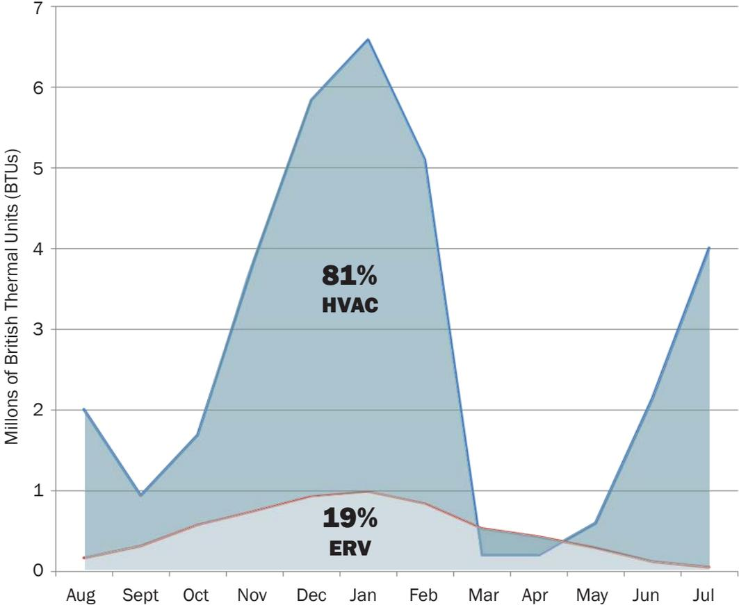
The New Norris House utilizes a Fantech energy recovery ventilator to achieve code required interior whole house and local ventilation. The unit provide fresh air and reduces the load of the heat and air system, saving energy and money.
