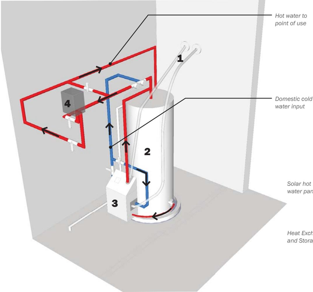
The New Norris House utilizes a solar hot-water panel system made by Enerworks. The system is supplemented by a small Eemax instantaneous water heater.
