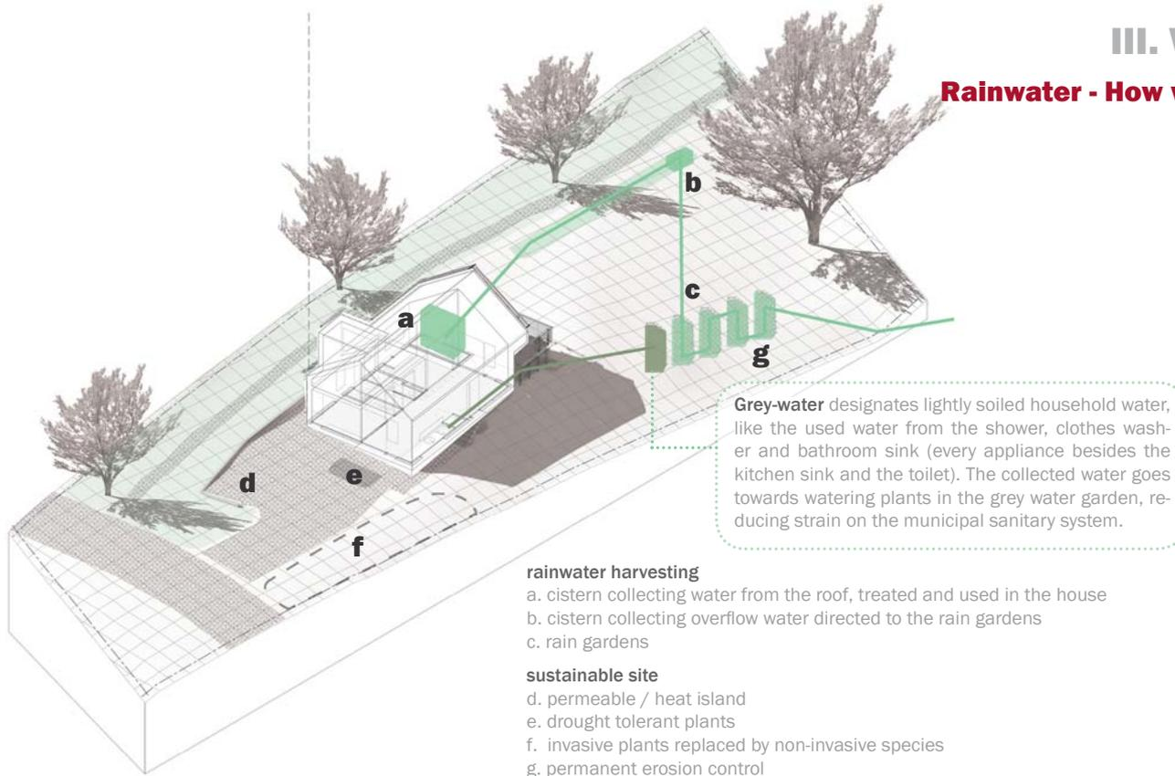
a. Cistern collects rainwater from the roof, the water is treated & used in the house for non-potable sources.
