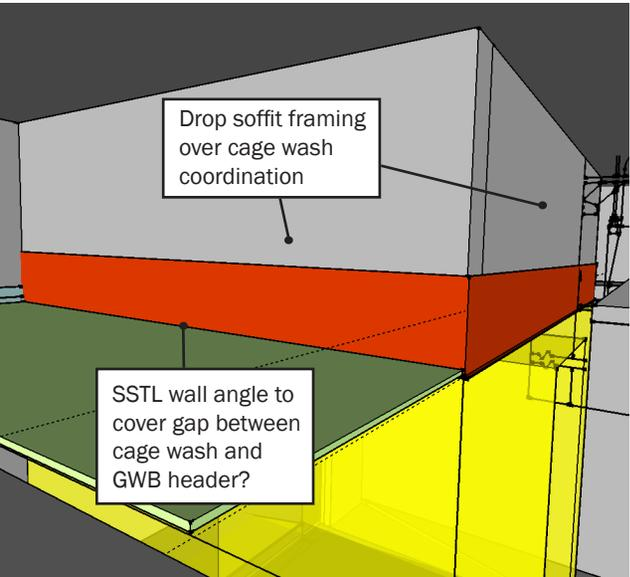
Drop soffit framing over cage wash coordination
